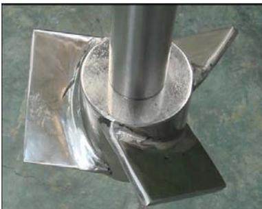
The 3-winged mixing propeller with 120 mm diameter is made of stainless steel. The propeller is polished.
